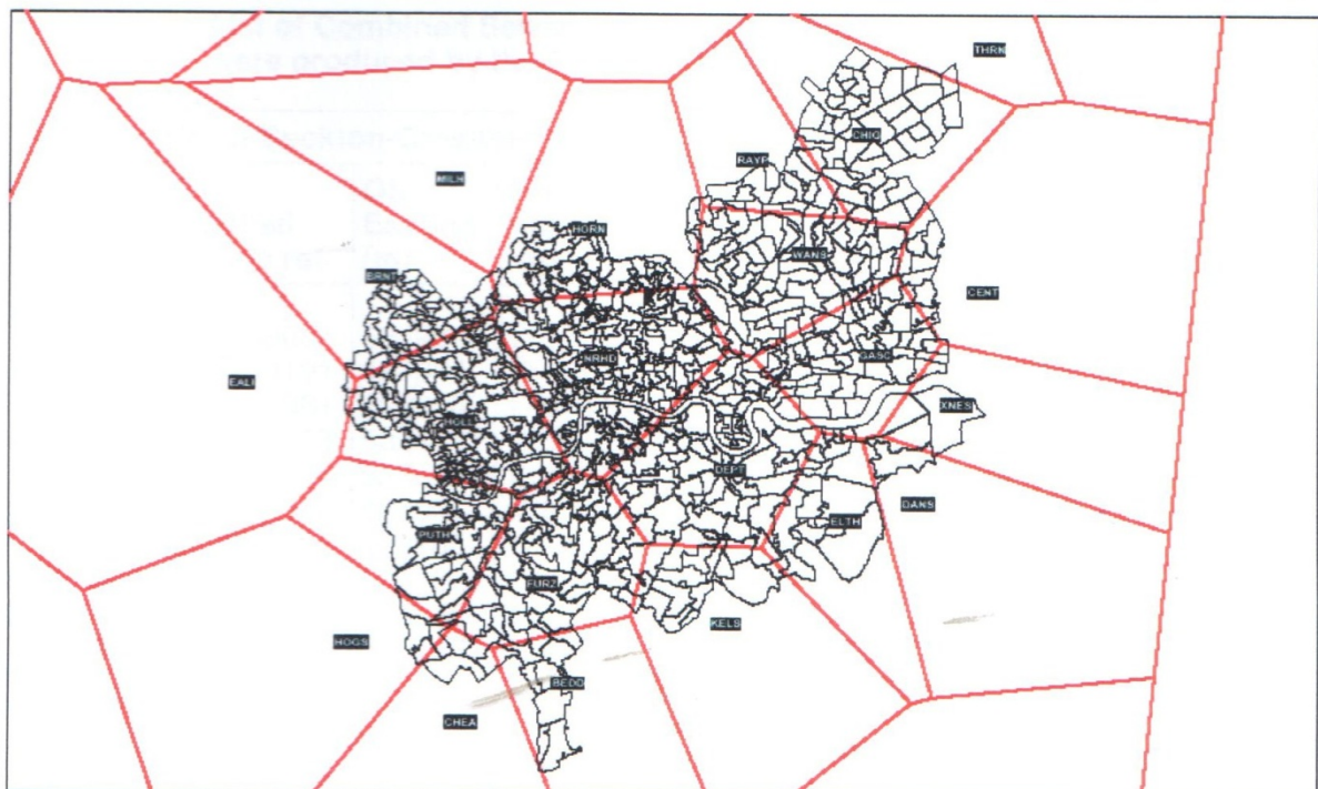
Figure 4.1 Allocation of rainfall gauges to sewer catchment areas
